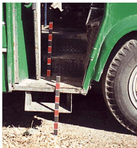
**Photo 5 Extra step installed under front door of *micro*, Mexico City**
