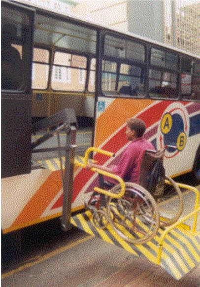
**High-floor buses** are more difficult to provide with wheelchair access. The approach used in Mexico City was to deploy 50 buses with lifts located in a dedicated rear door, deployed on six routes serving accessible metro stations. In South Africa similarly, equipped buses have been used in demonstration projects in peri-urban areas. These types of solutions may be appropriate where deteriorating road conditions are common.
