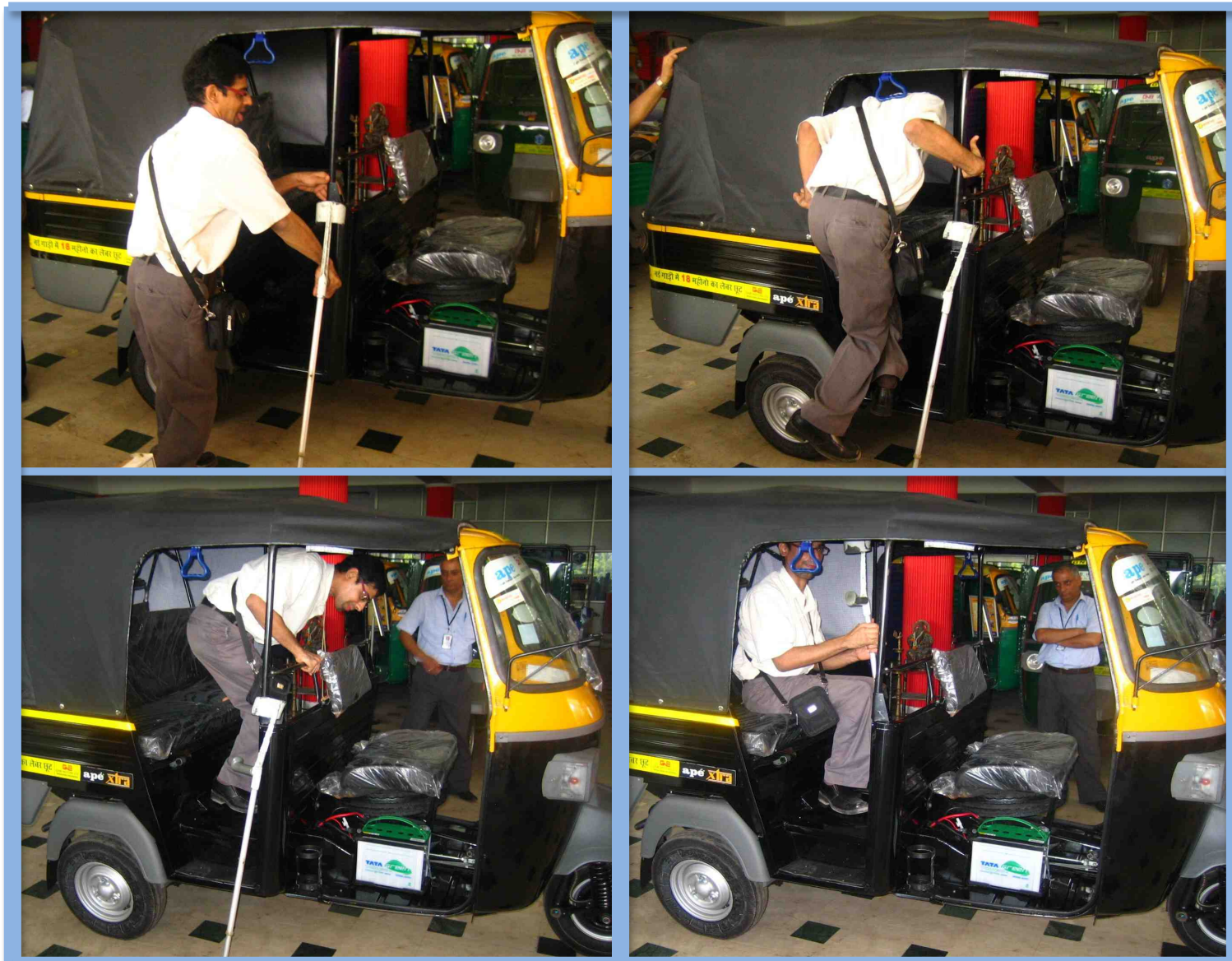
Manish Gupta of New Delhi illustrates the relative ease of entering a motorized low-floor autorickshaw, using existing vertical and horizontal handholds at a test session.
