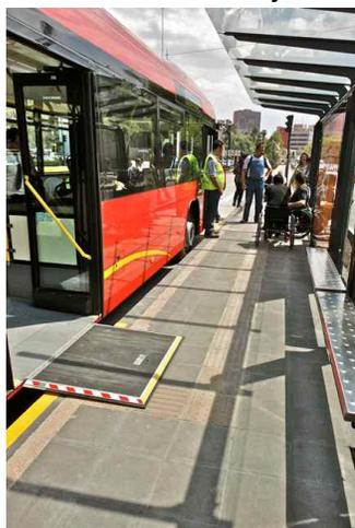
access including reduced gaps that wheelchair users can (usually) cross, or bridges to serve this purpose when needed, as shown in the photo at left on Line 5 through the city's historic district. Also note the tactile guideways. Other features include good color contrast, priority seating, and improved audio and text signage.
