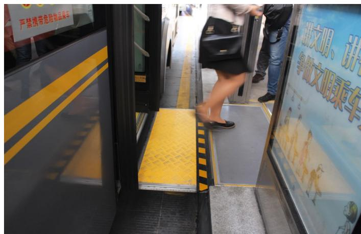
**A movable bridge, deployed from the platform of this bus rapid transit station in Yichang, China, eliminates the station-to-bus gap for all passengers. If the bridge deploys while the bus doors are opening, travel time would not be effected.** – ITDP photo forwarded by Gerhard Menckhoff
