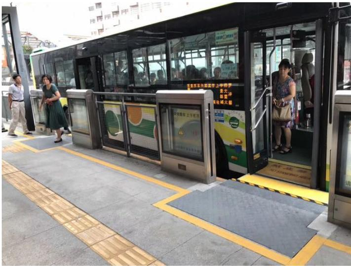
Gap filler deployed at Yichang BRT station
