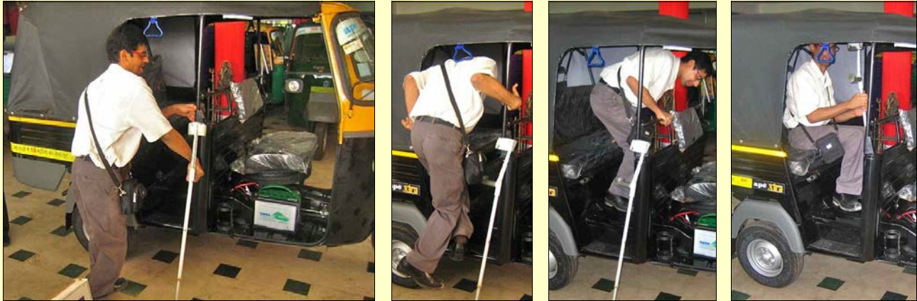
Manish Gupta of New Delhi illustrates the relative ease of entering a motorized low-floor auto-rickshaw, using vertical and horizontal handholds at a test session. - Photos by AEI
